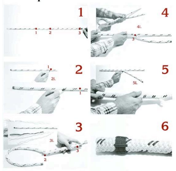
1. Measure one fid length plus one short fid length up the rope and make mark "1". Place mark "2" on the rope at two full fid lengths. Make mark "3" I full fid length plus 1 short fid length up from "2". The backsplice may be lengthened (useful for rigging "Kellerns" type grips) or could be shortened by lengthening or shortening mark "3" on the rope.
