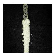
13) After making the required "half tucks", tape and cut each remaining strand to finish the splice. If desired, the strand ends may be "hot cut" and sealed to about 1/4 inch. The tail ends will pull closer to the braid when the splice is loaded and exercised. This retraction is normal unless it results in the loss of a "tuck".
