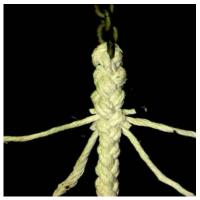
**11)** After making the required number of "full tucks", tape and cut away one strand from each strand pair. The tucks of these remaining single strands are referred to as "half tucks".
