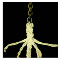
**10)** For this example, we are using spun polyester 8-plait. Table 1 requires 3 "full tucks". The picture at left shows the splice with 3 "full tucks" made on each strand pair.
