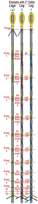
Tape over all fasten-offs and free tails to prevent snagging on sheaves and other rigging.
